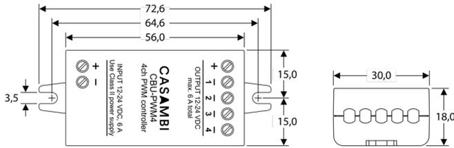
\*t<sub>c</sub> point is on bottom side • | Mounting hole diameter 3,5mm
