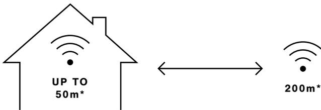
\*The wireless range of a Casambi unit is dependent on several factors; how it has been integrated into a luminaire, where it has been installed; taking into consideration surrounding obstacles such as walls and other building materials that may block signals.
